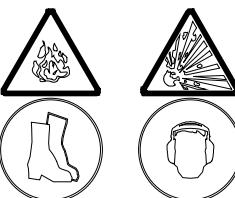
Cast material projections are given off during the welding process so due precautions must be taken. There must be a fire-extinguisher near to the working area. Do not keep inflammable material or explosives near to the working post. Prevent fire caused by sparks or slag. Use quality approved footwear for this type of operations. Use approved auditive protectors in case of too high noise.
